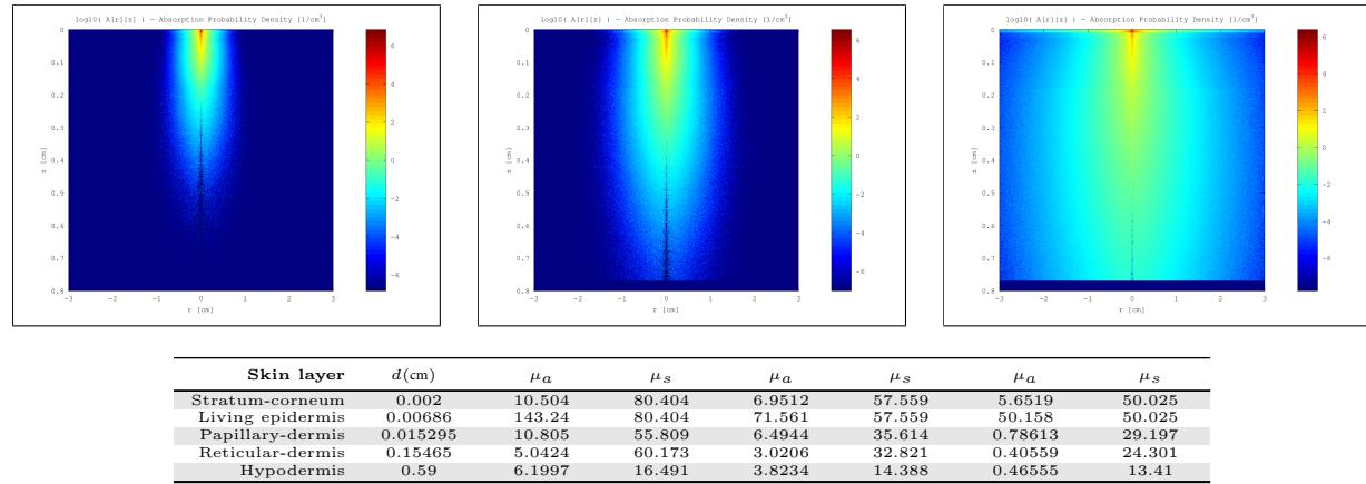
Figure 14: Top row: MonteCarlo simulations for 450nm, 550nm and 610nm. Bottom row: Resultant optical parameters ( $d$ ,  $\mu_a$ ,  $\mu'_s$ ) applying our skin aging model.
