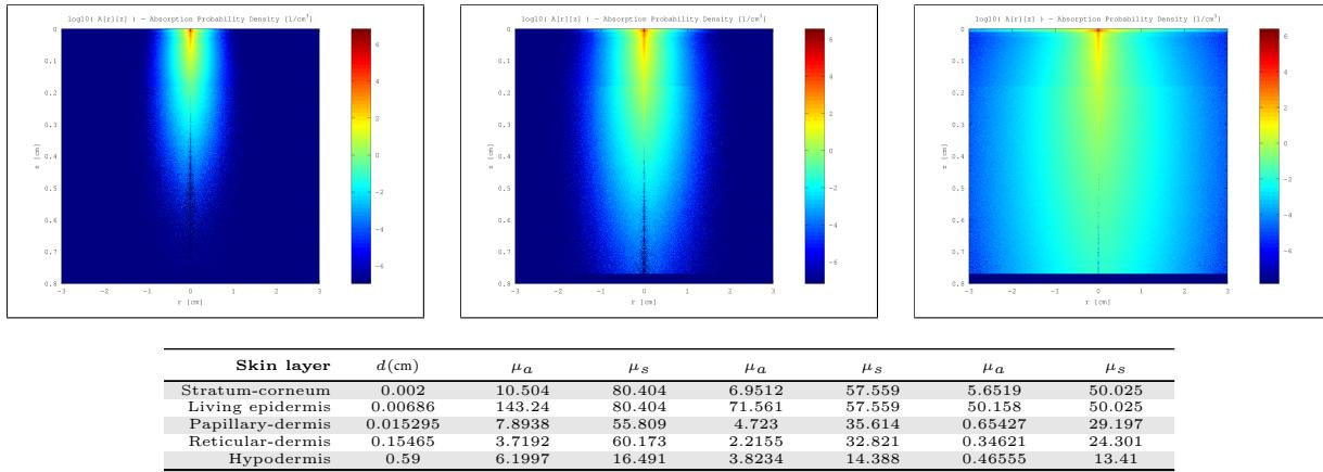
Figure 5: Top row: MonteCarlo simulations for 450nm, 550nm and 610nm. Bottom row: Resultant optical parameters ( $d$ ,  $\mu_a$ ,  $\mu'_s$ ) applying our skin aging model.
