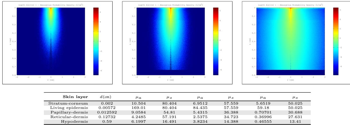
Figure 35: Top row: MonteCarlo simulations for 450nm, 550nm and 610nm. Bottom row: Resultant optical parameters ( $d$ ,  $\mu_a$ ,  $\mu'_s$ ) applying our skin aging model.
