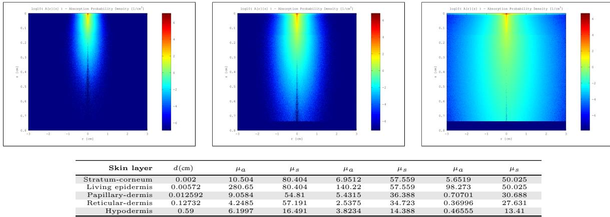
Figure 89: Top row: MonteCarlo simulations for 450nm, 550nm and 610nm. Bottom row: Resultant optical parameters ( $d$ ,  $\mu_a$ ,  $\mu'_s$ ) applying our skin aging model.
