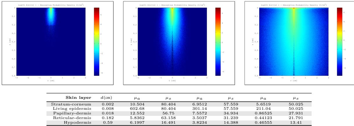
Figure 128: Top row: MonteCarlo simulations for 450nm, 550nm and 610nm. Bottom row: Resultant optical parameters ( $d$ ,  $\mu_a$ ,  $\mu'_s$ ) applying our skin aging model.
