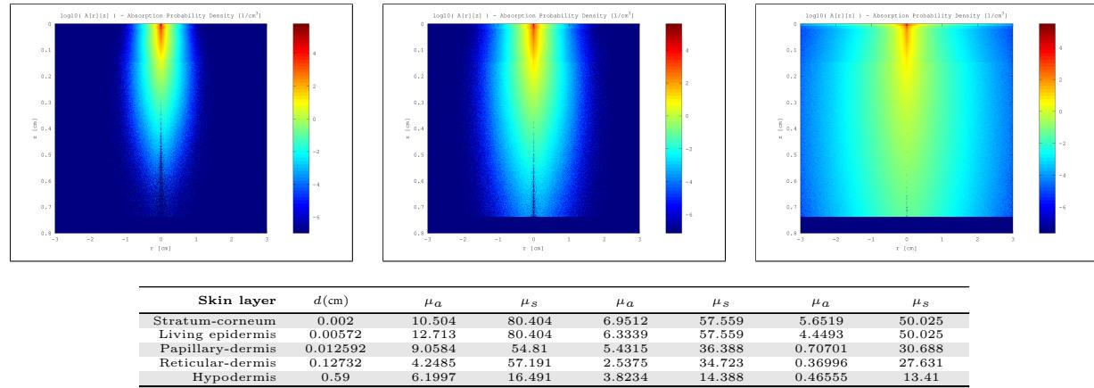
Figure 53: Top row: MonteCarlo simulations for 450nm, 550nm and 610nm. Bottom row: Resultant optical parameters ( $d$ ,  $\mu_a$ ,  $\mu'_s$ ) applying our skin aging model.
