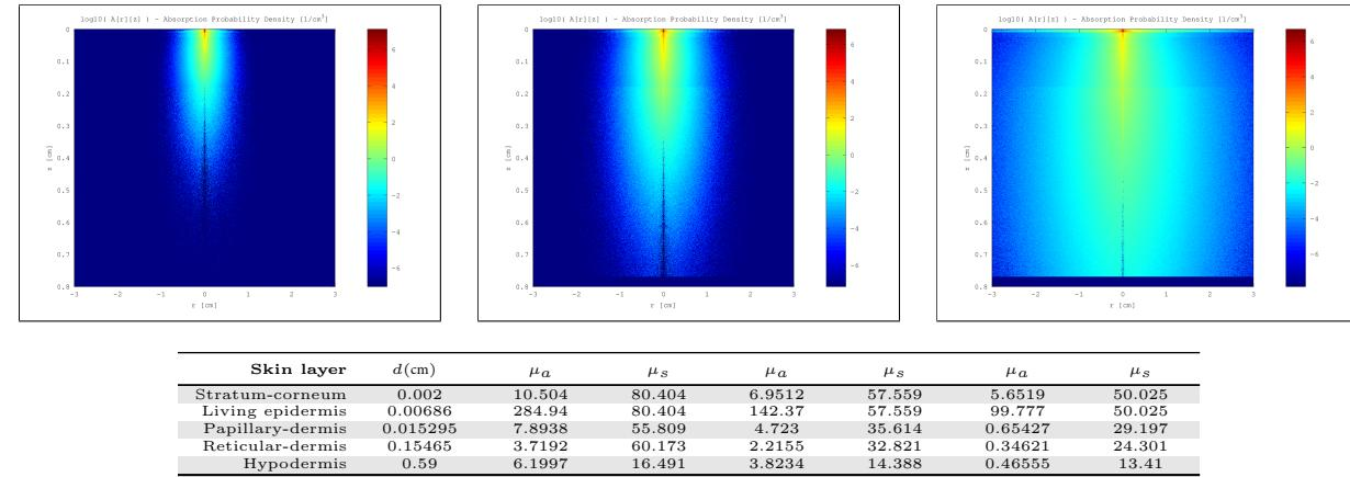
Figure 59: Top row: MonteCarlo simulations for 450nm, 550nm and 610nm. Bottom row: Resultant optical parameters ( $d$ ,  $\mu_a$ ,  $\mu'_s$ ) applying our skin aging model.
