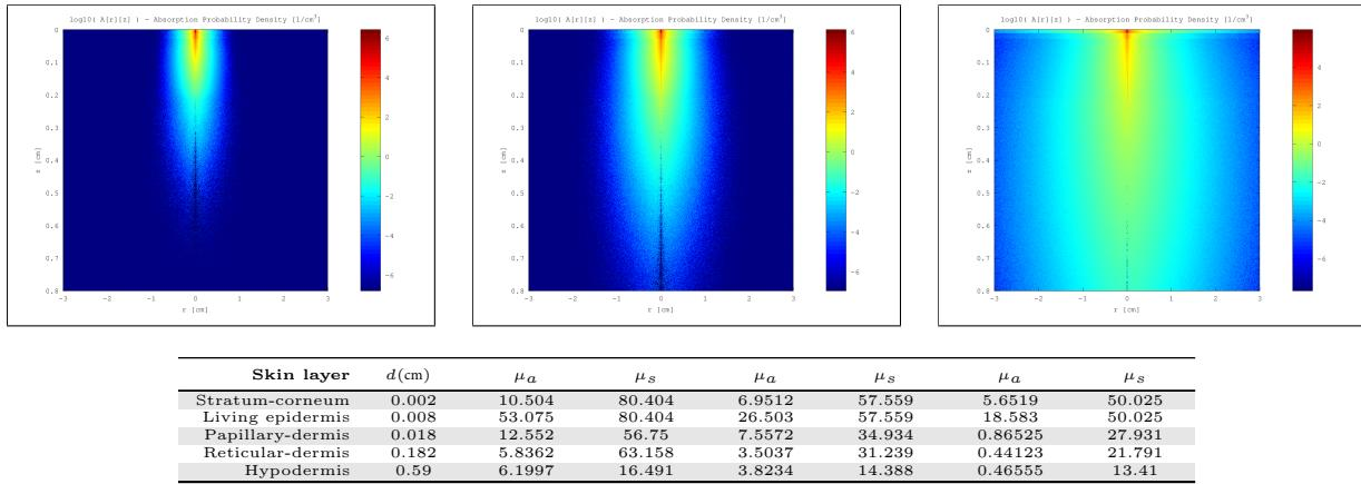
Figure 155: Top row: MonteCarlo simulations for 450nm, 550nm and 610nm. Bottom row: Resultant optical parameters ( $d$ ,  $\mu_a$ ,  $\mu_s'$ ) applying our skin aging model.
