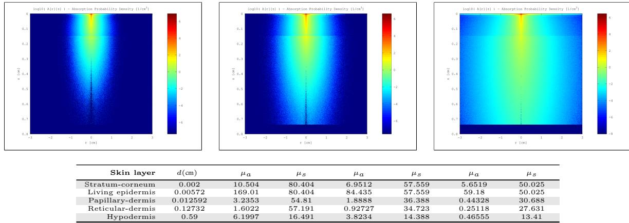
Figure 26: Top row: MonteCarlo simulations for 450nm, 550nm and 610nm. Bottom row: Resultant optical parameters ( $d$ ,  $\mu_a$ ,  $\mu'_s$ ) applying our skin aging model.
