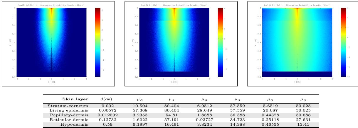
Figure 200: Top row: MonteCarlo simulations for 450nm, 550nm and 610nm. Bottom row: Resultant optical parameters ( $d$ ,  $\mu_a$ ,  $\mu'_s$ ) applying our skin aging model.
