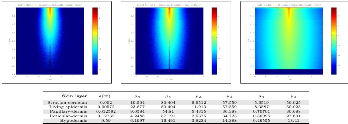
Figure 107: Top row: MonteCarlo simulations for 450nm, 550nm and 610nm. Bottom row: Resultant optical parameters ( $d$ ,  $\mu_a$ ,  $\mu'_s$ ) applying our skin aging model.
