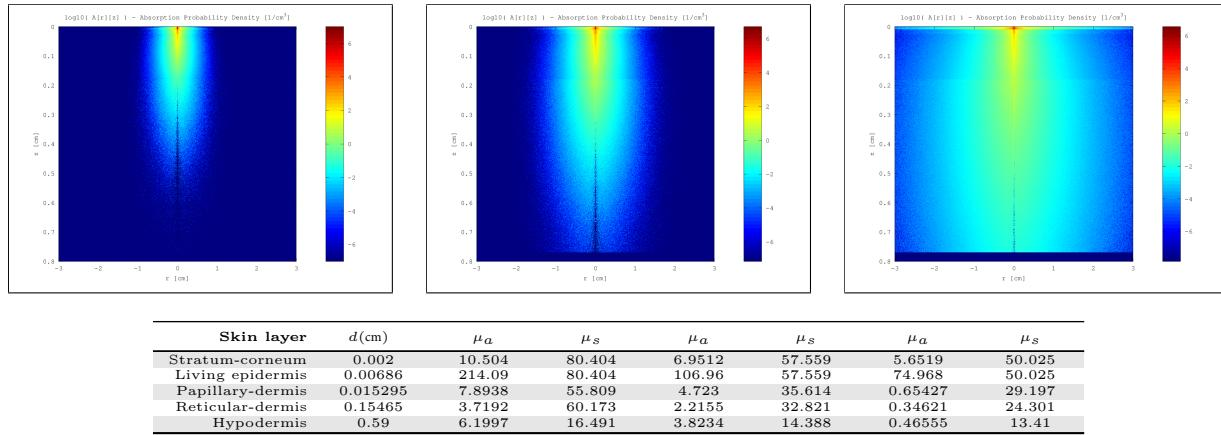
Figure 23: Top row: MonteCarlo simulations for 450nm, 550nm and 610nm. Bottom row: Resultant optical parameters ( $d$ ,  $\mu_a$ ,  $\mu_s'$ ) applying our skin aging model.
