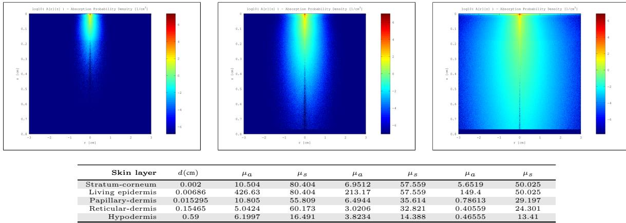
Figure 122: Top row: MonteCarlo simulations for 450nm, 550nm and 610nm. Bottom row: Resultant optical parameters ( $d$ ,  $\mu_a$ ,  $\mu'_s$ ) applying our skin aging model.
