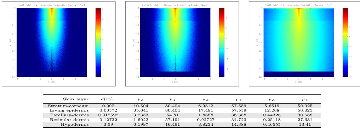
Figure 152: Top row: MonteCarlo simulations for 450nm, 550nm and 610nm. Bottom row: Resultant optical parameters ( $d$ ,  $\mu_a$ ,  $\mu'_s$ ) applying our skin aging model.
