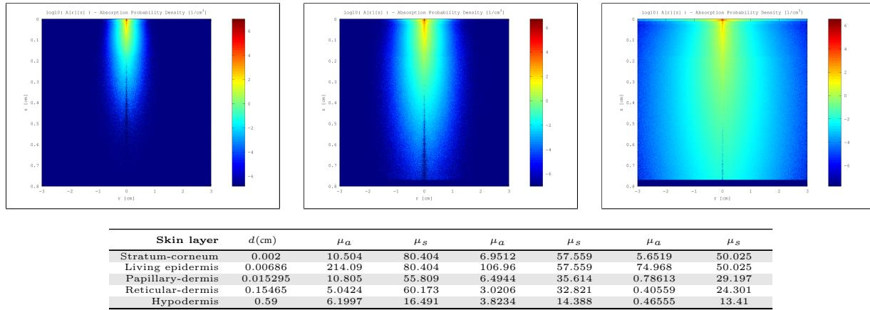
Figure 32: Top row: MonteCarlo simulations for 450nm, 550nm and 610nm. Bottom row: Resultant optical parameters ( $d$ ,  $\mu_a$ ,  $\mu_s'$ ) applying our skin aging model.
