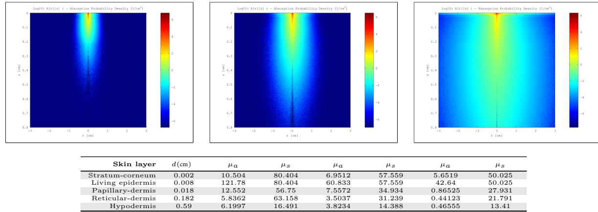
Figure 212: Top row: MonteCarlo simulations for 450nm, 550nm and 610nm. Bottom row: Resultant optical parameters ( $d$ ,  $\mu_a$ ,  $\mu'_s$ ) applying our skin aging model.
