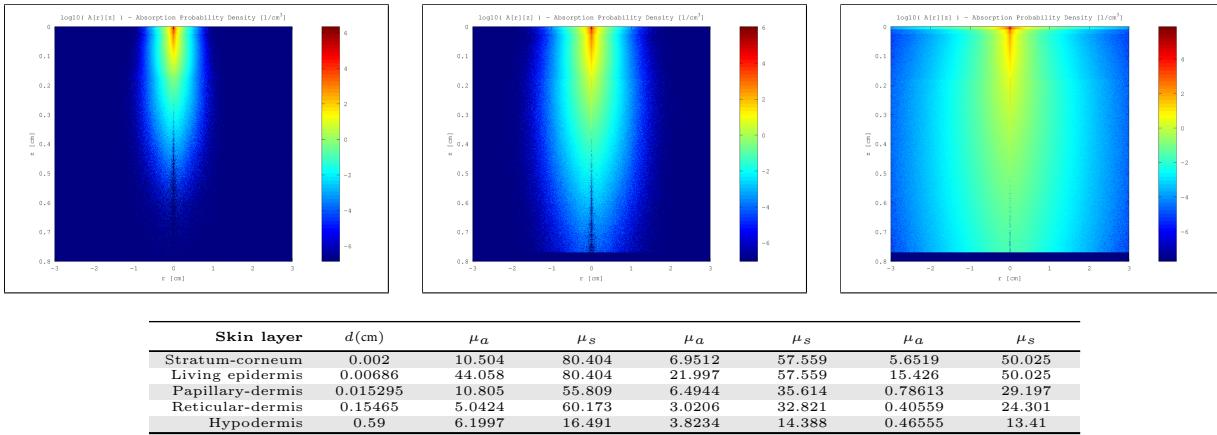
Figure 158: Top row: MonteCarlo simulations for 450nm, 550nm and 610nm. Bottom row: Resultant optical parameters ( $d$ ,  $\mu_a$ ,  $\mu'_s$ ) applying our skin aging model.
