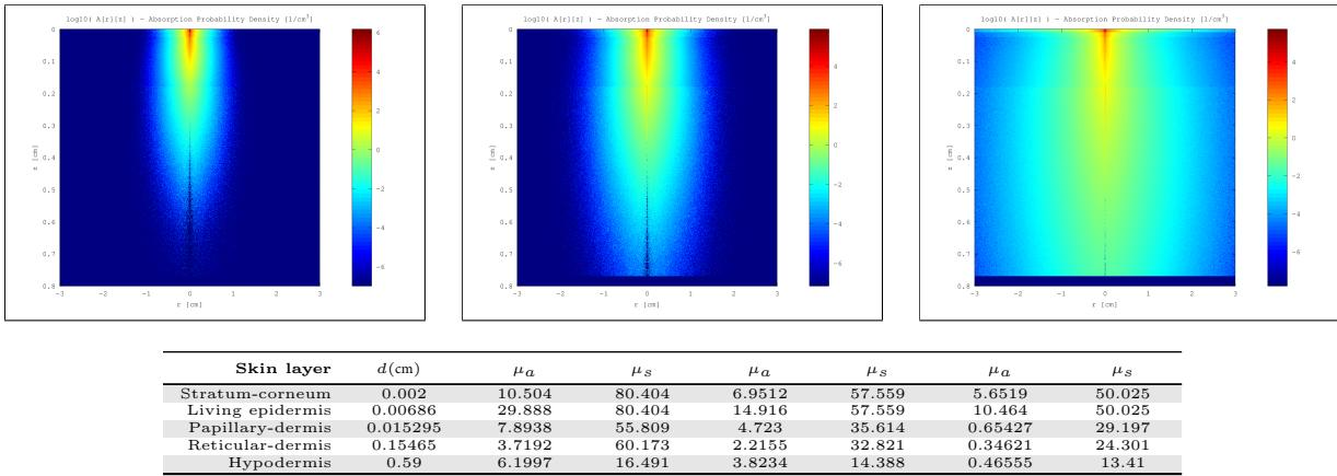
Figure 95: Top row: MonteCarlo simulations for 450nm, 550nm and 610nm. Bottom row: Resultant optical parameters ( $d$ ,  $\mu_a$ ,  $\mu_s'$ ) applying our skin aging model.
