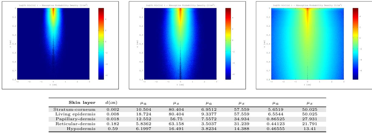
Figure 47: Top row: MonteCarlo simulations for 450nm, 550nm and 610nm. Bottom row: Resultant optical parameters ( $d$ ,  $\mu_a$ ,  $\mu_s'$ ) applying our skin aging model.
