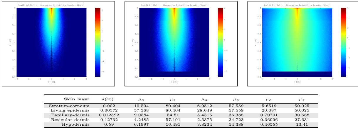
Figure 209: Top row: MonteCarlo simulations for 450nm, 550nm and 610nm. Bottom row: Resultant optical parameters ( $d$ ,  $\mu_a$ ,  $\mu'_s$ ) applying our skin aging model.
