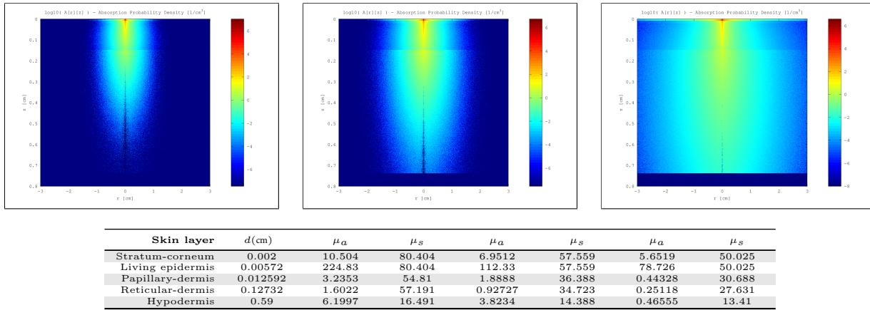
Figure 62: Top row: MonteCarlo simulations for 450nm, 550nm and 610nm. Bottom row: Resultant optical parameters ( $d$ ,  $\mu_a$ ,  $\mu'_s$ ) applying our skin aging model.
