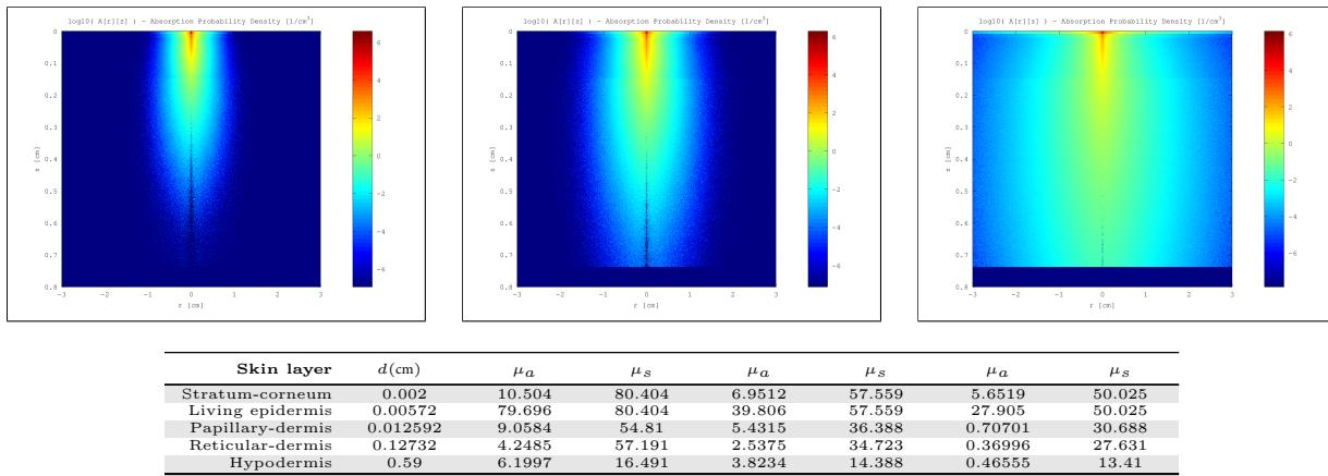
Figure 227: Top row: MonteCarlo simulations for 450nm, 550nm and 610nm. Bottom row: Resultant optical parameters ( $d$ ,  $\mu_a$ ,  $\mu_s'$ ) applying our skin aging model.
