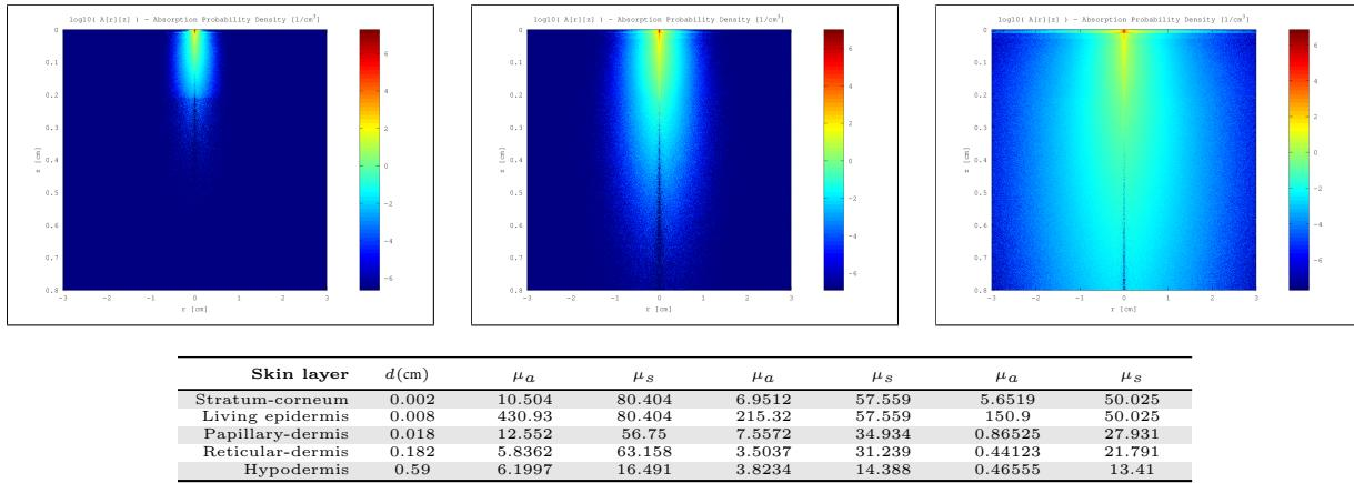
Figure 83: Top row: MonteCarlo simulations for 450nm, 550nm and 610nm. Bottom row: Resultant optical parameters ( $d$ ,  $\mu_a$ ,  $\mu'_s$ ) applying our skin aging model.
