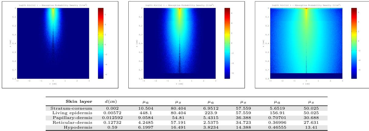
Figure 176: Top row: MonteCarlo simulations for 450nm, 550nm and 610nm. Bottom row: Resultant optical parameters ( $d$ ,  $\mu_a$ ,  $\mu_s'$ ) applying our skin aging model.
